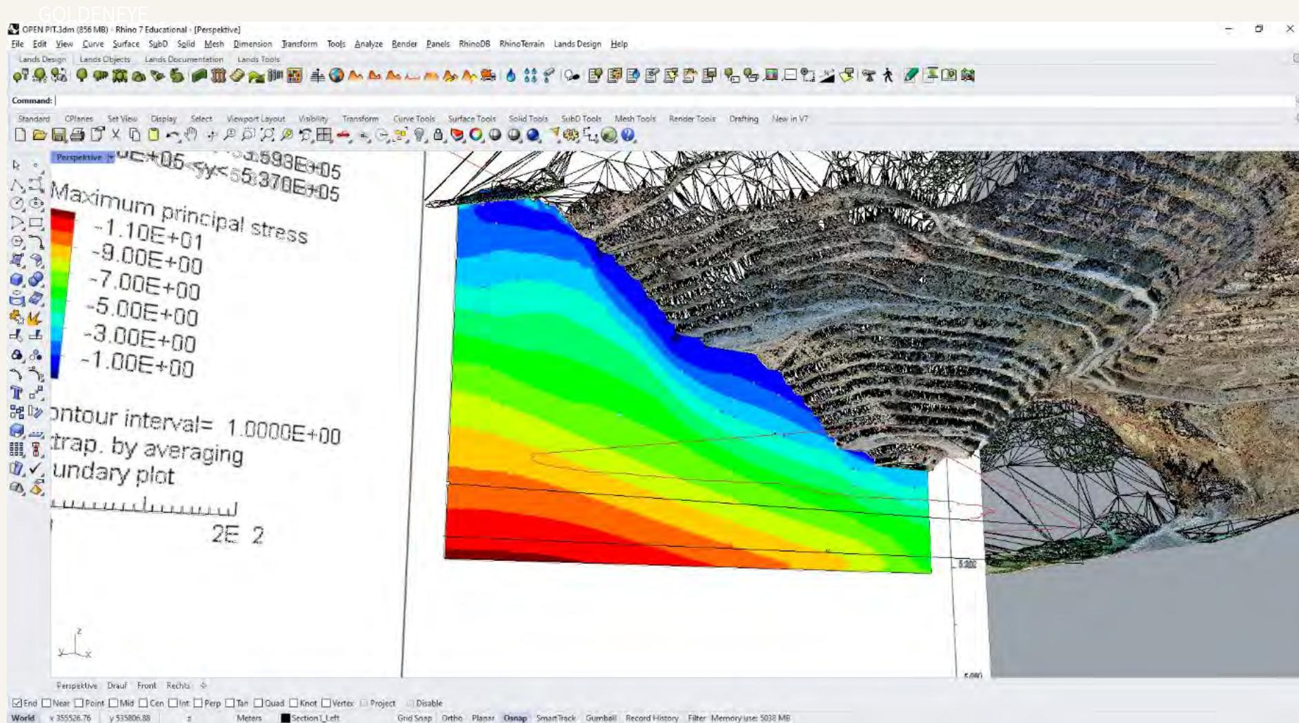
*Figure 7: Attached numerical simulation results to the real geometry*
