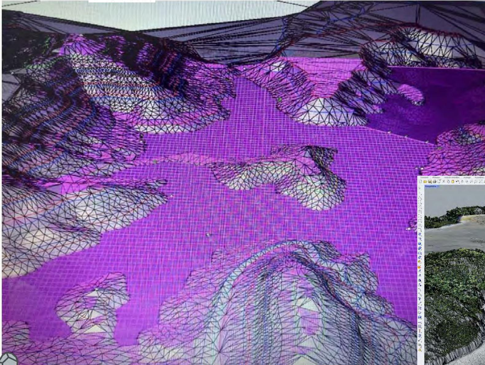
High 3D resolution elevation model of Valea Sesei Tailing Pond – Volume at 708m asl (68.036.554 m<sup>3</sup>)
