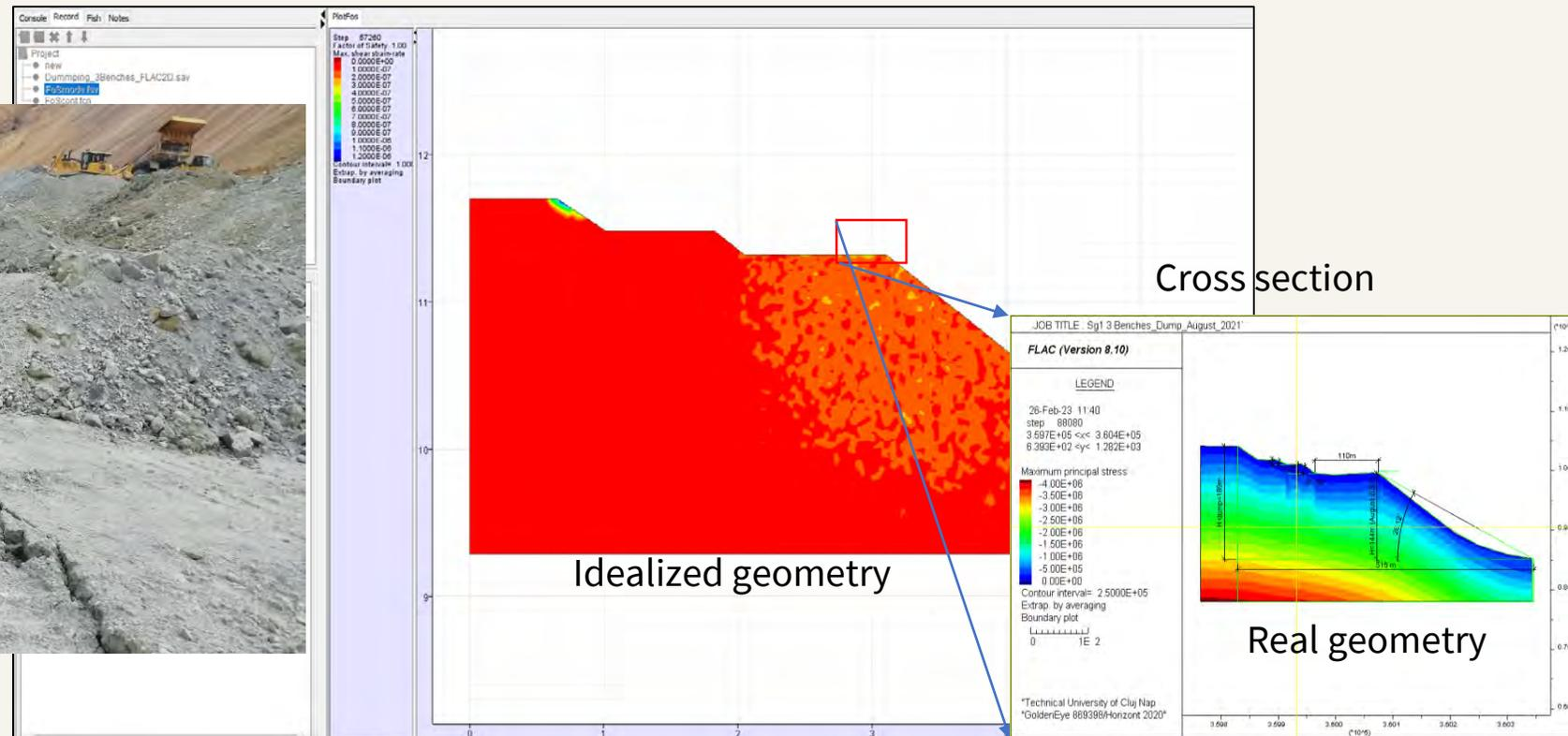
Example of factor of safety prediction over waste dump cross section at Rosia Poieni
