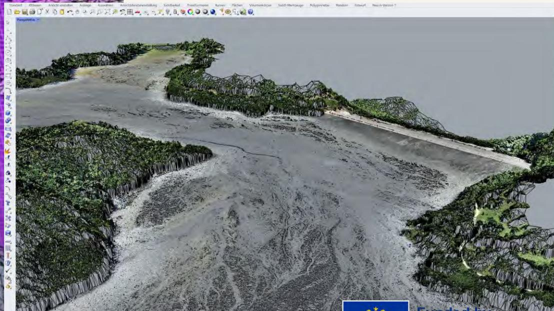
High 3D resolution elevation model of Valea Sesei Tailing Pond – Volume at 725m asl (116.743.583 m<sup>3</sup>)
