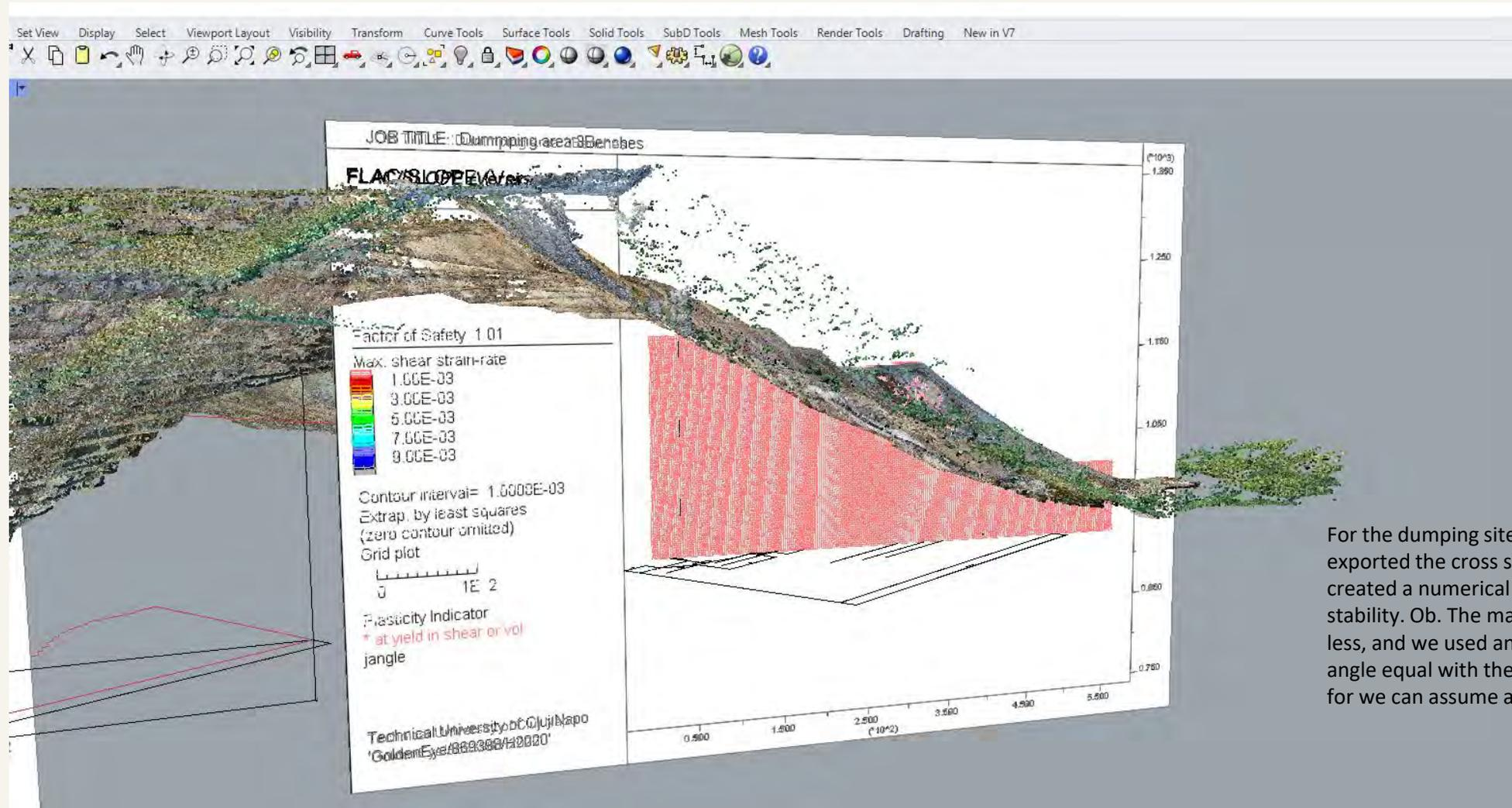
For the dumping site area was also exported the cross section of it and created a numerical simulation of its stability. Ob. The material is cohesion less, and we used an internal friction angle equal with the slope angle, there for we can assume a FoS by the limit.
