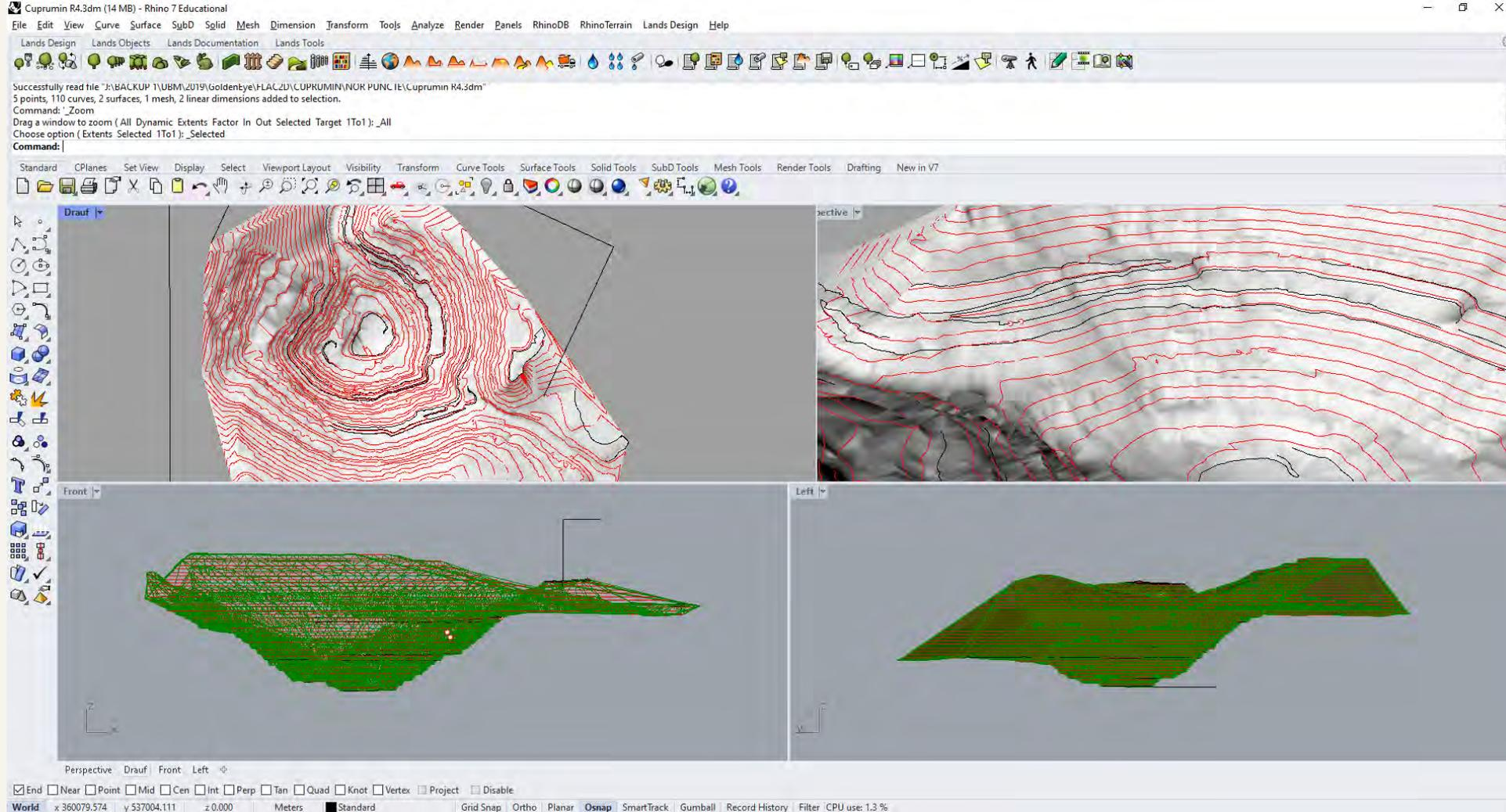
Figure 2: Triangulated surface of the Open Pit-a real scale of 1:1 of the Open Pit
